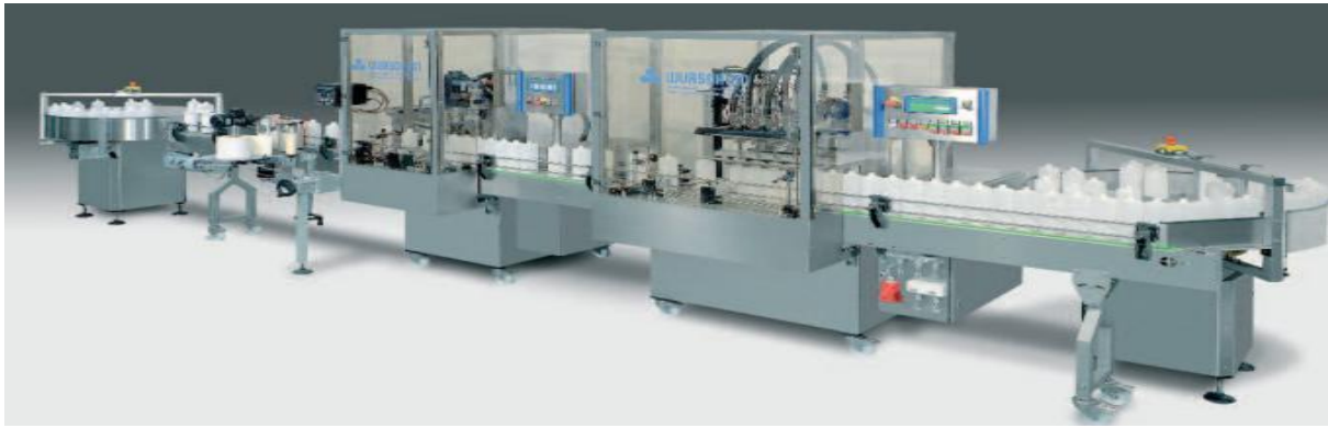
Figure 2 - Automatic bottling line
